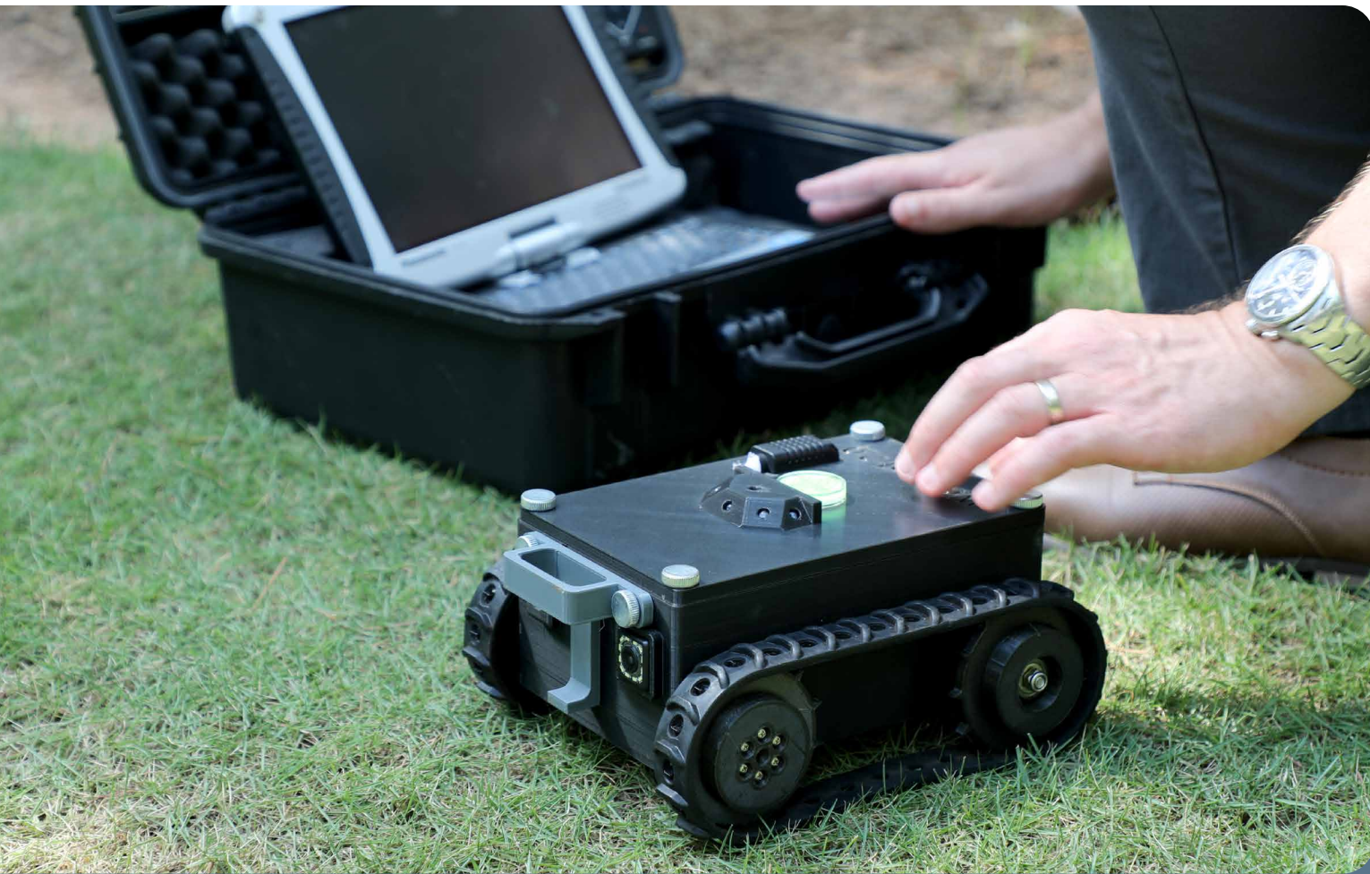
The WomBot, designed in collaboration with a robotics engineer, allows researchers to gather data inside wombat burrows. Driven using a Gameboy-type controller, it's equipped with sensors and a thermal camera. (Photo: Allyson Mann)
