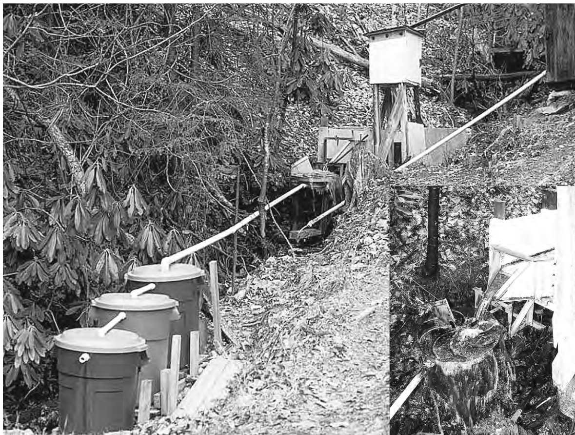
PLATE 1. Field apparatus for independent measurement of stream discharge and export of fine particulate organic matter (FPOM) from the reference stream (C53) at Coweeta Hydrologic Laboratory, North Carolina, USA. Discharge is measured by a calibrated bubble flow-meter in the H-flume. A flow-proportional sample of streamwater exiting the flume is captured by the hollow blade (4-mm aperture) of a Coshocton wheel sampler (see inset). The continuous sample flows to a series of three settlement barrels (main photo). Export of FPOM to the barrels was quantified every ~14 d in this study and subsequently corrected for settlement efficiency and proportion captured. The coarse particulate organic matter trap (4-mm mesh) is immediately upstream of the flume. An identical system was used at the terminus of the treatment stream (C54). Photo credits: S. L. Eggert (main photo) and Deanna Connors (inset).
